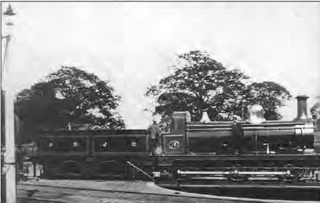
Fowler 0-6-0 No. 19, with Stirling-type cab, stands with the loco on the turntable and the tender off, in 1904. Note the yard lamp next to the shed roads. J Dyett. Courtesy Robin Atthill Collection
