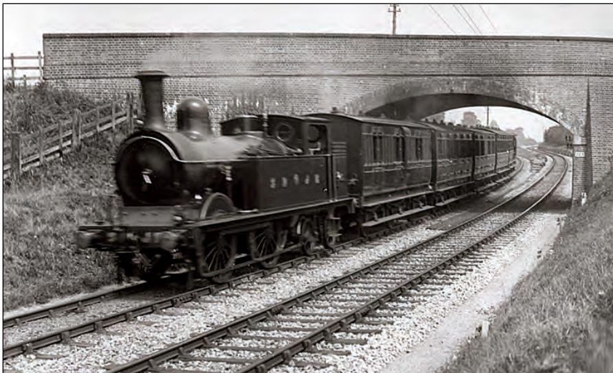
Johnson 0-4-4 tank and Bath train come off the Wimborne loop under Bridge 223 east of Corfe Mullen Junction, circa 1910. The Junction here was created in 1905, before that the two bi-directional single lines connected east of Bailey Gate Station.
