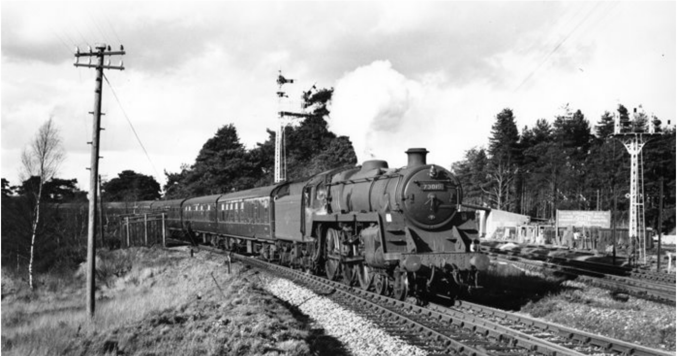
BR Standard Class 5 4-6-0 locomotive No. 73019 comes off the single line from Corfe Mullen and approaches the junction at Broadstone with the Down 'Pines Express'. The 1903 doubling scheme envisaged a siding where the photographer is standing. 31 March 1962. [Photo by Mike Fox/S&DRT collection, ref. WSHSD_2016_42_35.]
